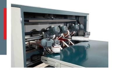
This machine is used during the carcass preparation at the beginning of the mattress assembling process. In other words, the machine is used to reduce the width and height of foam, latex, bonnell spring and pocket spring mattresses and insert them into a cover easily and quickly.
