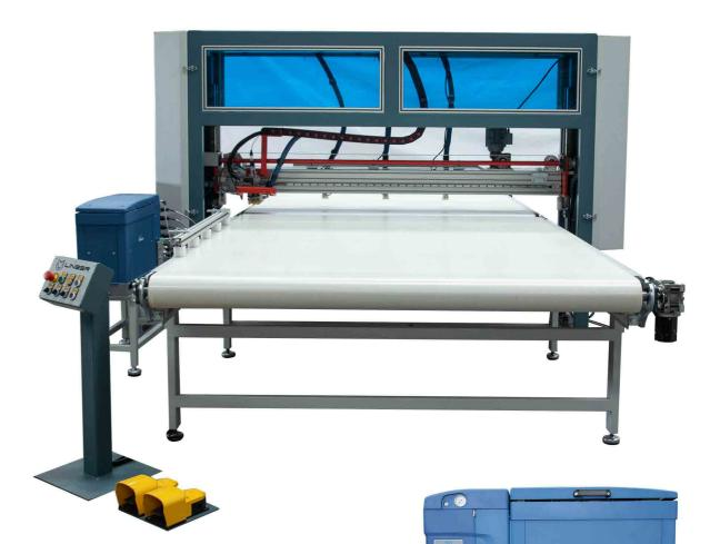
NOTE: The ROBATECH or NORDSON Hotmelt system is used in the glue bridge. 3 fixed and 3 Moving, total 6 guns /24 nozzles are used. Tank capacity: 30lt. Tank capacity can vary according to our client's request
