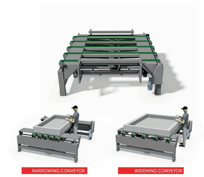
LM-MPL-CAW/11000 **TECHNICAL DATA** Conveyor Size W:2350 mm L:2600 mm H:1200mm Conveyor Weight 1500 kg 900 mm Conveyor Height Capacity 1 mattress/45 sec Max. Mattress Size W:2000 mm L:2250 H: 500 mm Min. Mattress Size W:700 mm L:1800 mm H:100 mm 150 kg Max. Mattress Weight Dynamic system **Ball Screw** 380 VAC (III+N+TT) Electric Air Pressure 6-8 bar Power Total:1.5kW **CE Certificate** Yes
